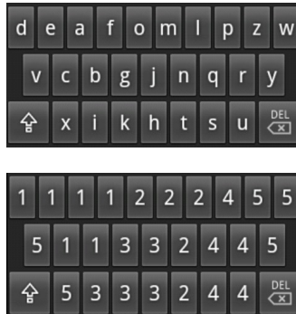
Figure 5: Optimized English mobile keyboard generated with a population of 5000 over 20000 generations. This layout has an estimated typing speed of 84 WPM and an average distance of 1.43 keys between two characters in the same group. The lower diagram shows the group number of each character.
