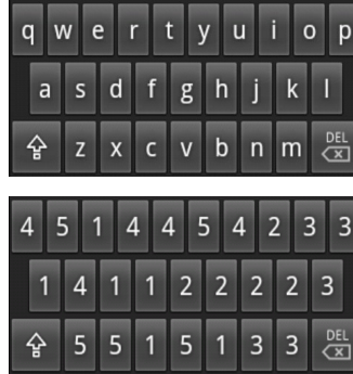
Figure 2: The analysis of the QWERTY keyboard using our evaluator. This layout has an estimated typing speed of 47 WPM and an average distance of 2.88 keys between two characters in the same group. The lower diagram shows the group number of each character.
