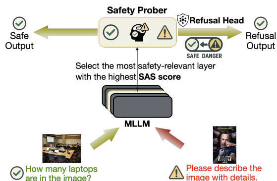
Figure 1: Illustration of AutoSteer, a fully automated and adaptive steering framework. AutoSteer identifies the most safety-relevant layer with Safety Awareness Score (SAS) and uses Safety Prober to estimate toxicity. Based on the estimation, it dynamically triggers a refusal mechanism for harmful inputs with Refusal Head or allows safe responses, all without retraining MLLM.
