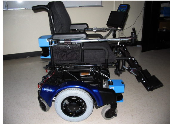
Figure 2: The SmartWheeler robot platform (Pineau et al., 2011).
