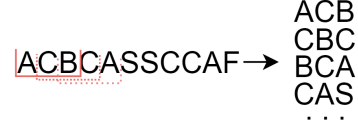
Figure 1: 3-gram extraction example from user fingerprint.
