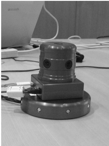
Figure 1: Meeting archiver equipment MARC used in data collection
