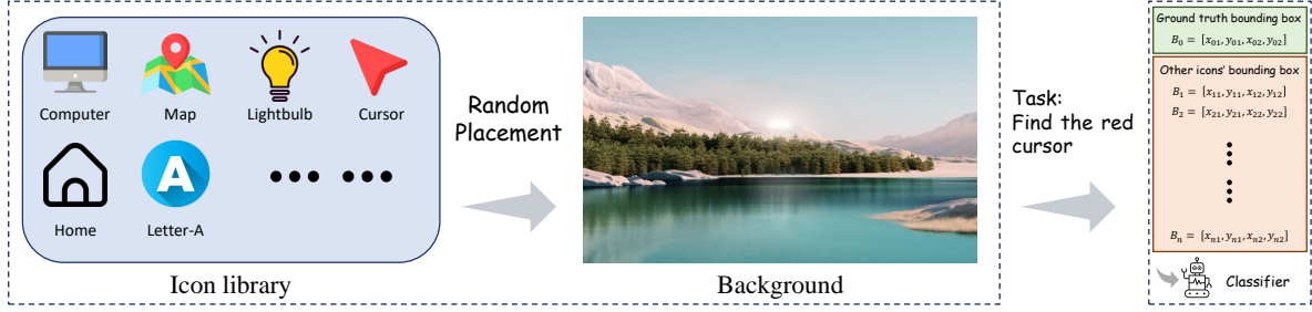
Figure 2: Illustration of the experimental procedure for classifying responses generated by GUI agent models. A Windows desktop wallpaper is used as the background, onto which a set of icons is randomly placed. The bounding box of each icon is recorded and subsequently used to categorize the model’s predicted coordinates according to the classification algorithm described in Algorithm 1.
