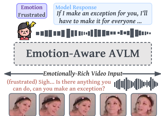
Figure 1: Our Audio-Visual Language Model (AVLM) perceives an audio-visual input, determine the emotion of the speaker and generate an expressive response.
