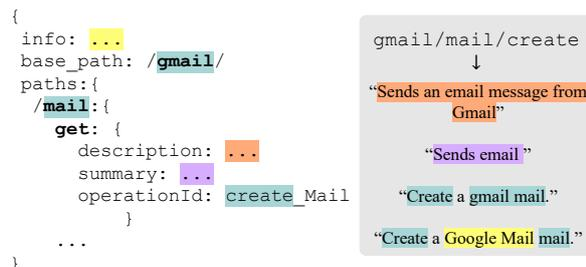
Figure 2: Synthetic utterance generation from the OpenAPI specification.
