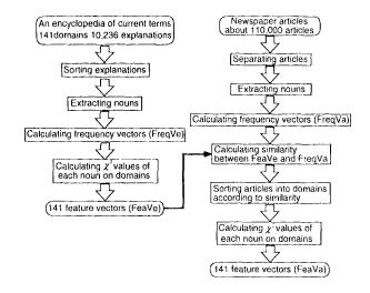
Figure 2: Calculating feature vectors
