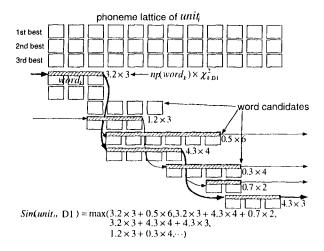
Figure 3: Calculating similarity between  $unit_i$ and D1
