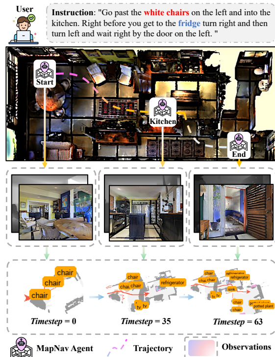
Figure 1: Illustration of our Annotated Semantic Map (ASM). At each timestep, MapNav agent leverages egocentric observations to capture semantic objects and assign explicit textual labels to key regions, creating the ASM for the current moment. ASM provides information such as physical obstacles, explored regions, the agent’s current position, trajectory and semantic objects.
