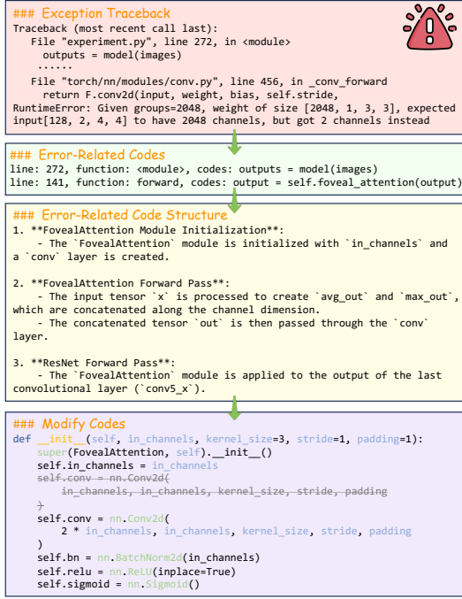
Figure 3: Debugging with traceback-guided local code structure.
