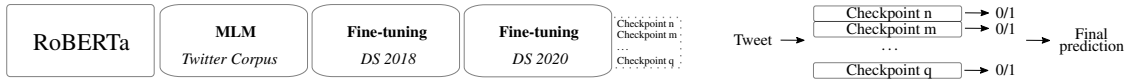
Figure 1: Our training (left) and test (right) pipeline for the Ensemble MLM model.
