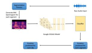
Figure 2: Visual Representation of the VGGish-based model.
