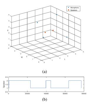
Figure 1: Experimental Setup. (a) Four microphones and two speakers (Table 1) in a room of dimension  $5 \times 5 \times 5$  (we assume a cuboid so that we are consistent with (Raikar et al., 2020)), (b) A sample  $\lambda(t)$  where the x-axis represents the time (expressed in samples) and y-axis can take a value of 1 or 2 depending on who is speaking. Note that at any given time only one of the speaker is speaking (no overlap).
