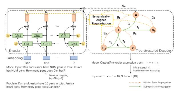
Figure 2: An overview of our SAU-Solver. When a problem preprocessed by number mapping and replacement is entered, our problem encoder encodes the problem text as context representation. Then our equation decoder generates an expression tree explicitly in pre-order traversal for the problem according to the context representation. Finally, infix traversal and inverse number mapping are applied to generate the corresponding equation.
