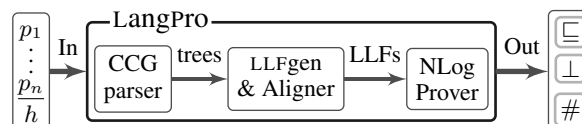
Figure 1: LangPro checks whether a set of premises p_1, \dots, p_n entails ( \sqsubseteq ), contradicts ( \perp ) or is neutral ( \# ) to a hypothesis h .
