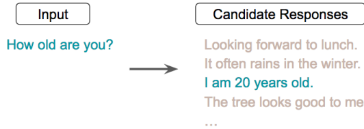
Figure 2: The conversational response selection problem attempts to identify the correct response from a collection of candidate responses. We train using batch negatives with each candidate response serving as a positive example for one input and a negative sample for the remaining inputs.
