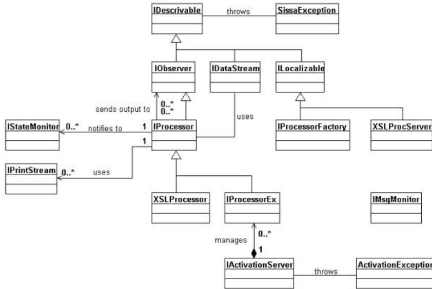
Figure 1: The UML diagram of the SiSSA IDLs.
