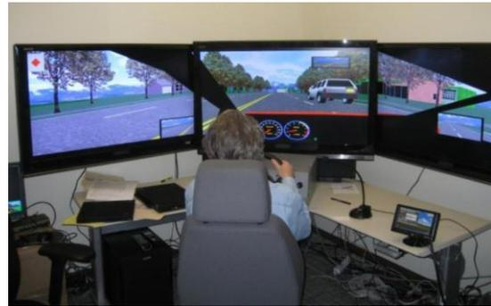
Figure 1. Driving simulator setup.
