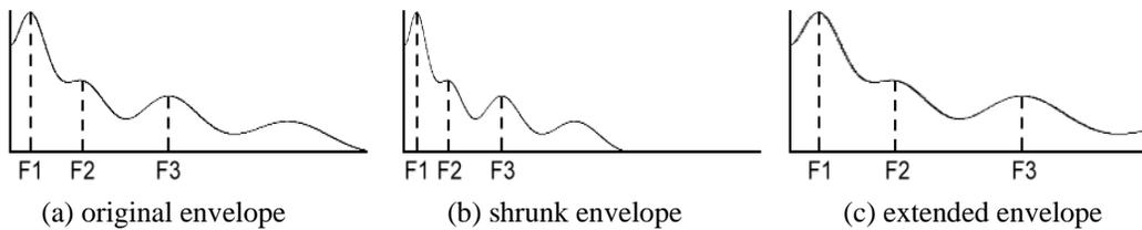
**Figure 12. The scaling of an example spectral envelope.**
