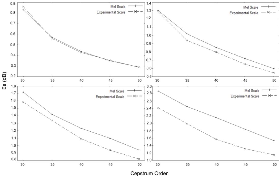
**Figure 10.** Approximation errors measured for our frequency conversion and mel-frequency conversion in the four frequency ranges: 0 ~ 2,000Hz (upper left), 0 ~ 4,000Hz (upper right), 0 ~ 6,000Hz (bottom left), and 0 ~ 11,025Hz (bottom right).
