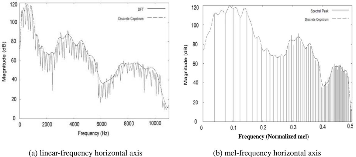
**Figure 8. Spectral envelopes approximated in mel-frequency scale.**
