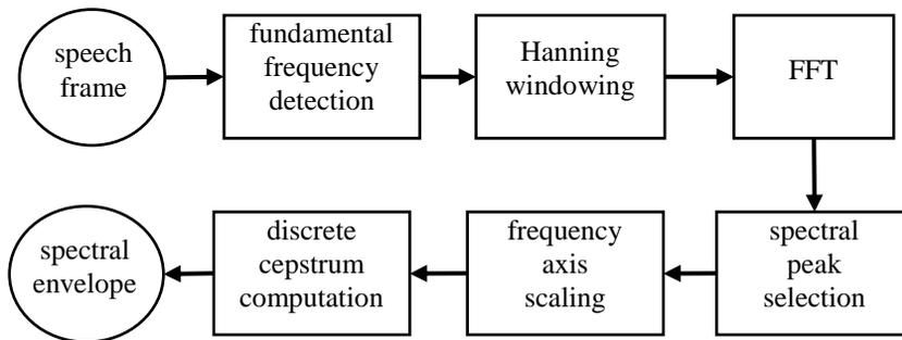
**Figure 2. Main flow of the spectral-envelope estimation scheme.**
