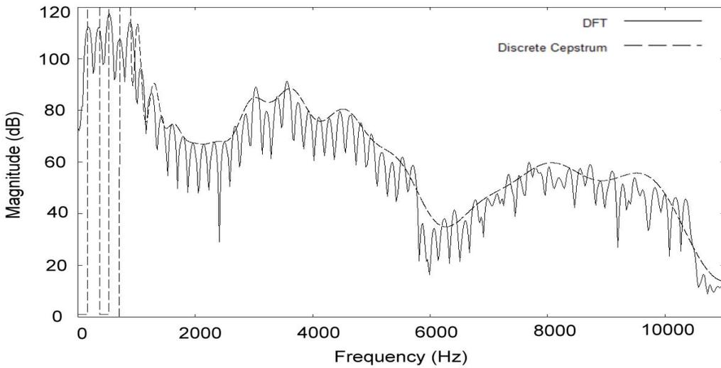
**Figure 3. A spectral envelope computed with 40 non-regularized discrete cepstrum coefficients.**
