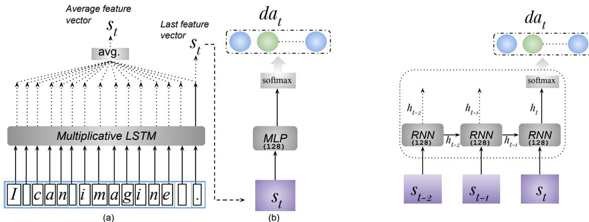
Figure 1: (a) Multiplicative LSTM (mLSTM) character-level language model to produce the sentence representation  $s_t$ . The character-level language model is pre-trained and produces the feature (hidden unit states of mLSTM at the last character) or average (average of all hidden unit states of every character) vector representation of the given utterance. (b) Utterance-level classification using a simple MLP layer with a *softmax* function (our baseline model).
