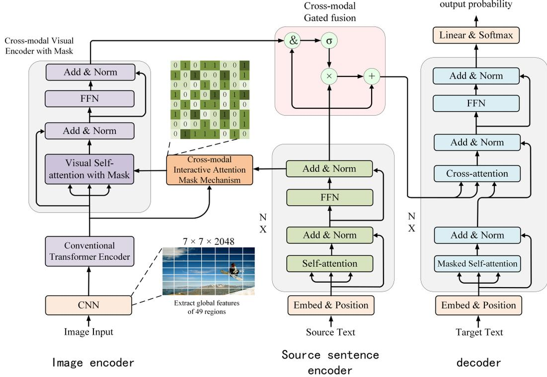
Figure 2: The overview of our proposed model, which consists of four components: (a) the image encoder to encode visual information with cross-modal interactive attention mask mechanism based on Transformer encoder; (b) the source sentence encoder to encode textual information; (c) the cross-modal gated fusion module to fuse helpful visual features and textual features; (d) the decoder to generate target translation conditioned on encoded textual features with helpful visual information;
