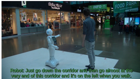
Figure 9: Robot describing a route to a human in a mall using the SSR and the associated algorithms. The sentence in green is the explanation of the route verbalized by the robot from the SSR representation: "just go down the corridor and then go almost at the very end of this corridor and it's on the left when you walk".
