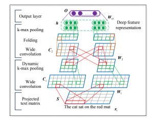
Figure 2: Dynamic convolutional neural network used for extracting deep feature representation
