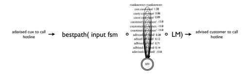
Figure 2: Illustration of the normalization technique using finite state transducers. The unknown words in the input are preserved in the output.
