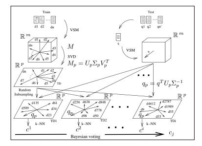
Figure 1: Fundamental steps of the proposed approach.  $\mathbb{R}^{m}$  is the original vector space,  $\mathbb{R}^{p}$  is the reduced dimensional space where vectors are projected. The multi-classifier is composed of several k-NN classifiers.  $c_{j}$  is the final classification label for testing case q.
