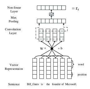
Figure 2: The architecture of CNN/PCNN used for sentence encoder.
