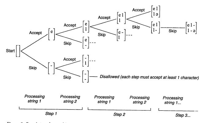
Figure 2: Search tree factored into 2-way branchings with a disallowed state at each step. This tree generalizes to handle more than 2 strings.
