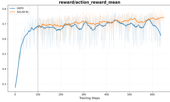
Figure 5: Mean action reward during training. GRPO collapses in later stages, whereas SOLAR-RL improves monotonically and converges.
