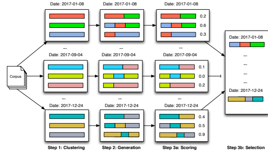
Figure 1: A graphical overview of our system. We can see that not all clusters are included in the timeline.
