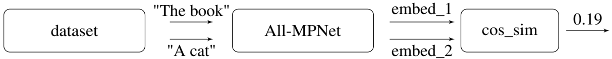
Figure 1: Block diagram of our proposed approach. Given a sample from the dataset, the first sentence is encoded with an All-MPNet embedding for generating an embedding vector as output. Also, the second sentence in the sample is encoded in the same way. Then the two embedding vectors are compared using cosine similarity to produce the final prediction on the semantic similarity of the two sentences.
