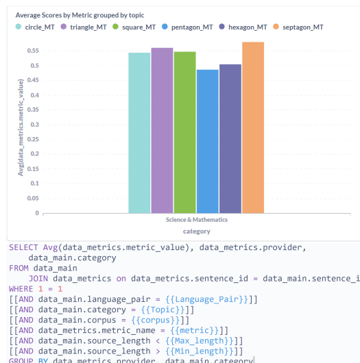
Figure 1: Sample plot with associated SQL statement. Optional conditions are put between square brackets.
