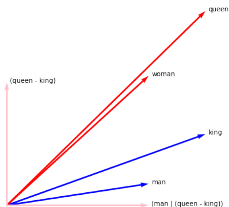
Figure 1: Projections of w_{king} , w_{queen} , w_{man} , w_{queen} - w_{king} and w_{man} projected away from w_{queen} - w_{king} . Both the vector arithmetic and the visualisation were done using the whatlies . The support for arithmetic expressions is integral in whatlies because it leads to more meaningful visualisations and concise code.
