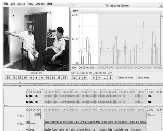
Figure 2: Screenshot of the annotation client interface, with video, time-aligned textual annotations, and time series displays.
