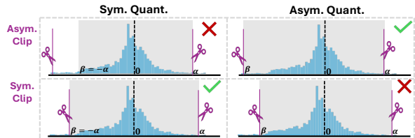
Figure 4: Comparison between asymmetric and symmetric weight clipping w.r.t. asymmetric/symmetric quantization. After weight clipping, we obtain the final range of tensor to quantize as depicted in the solid gray box related to asymmetric/symmetric quantization.
