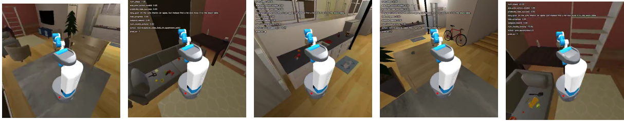
Start scene: navigate to sofa Scene 2: pick lid, pick box, navigate to left counter Scene 3: pick lego, pick strawberry, navigate to brown table Scene 4: pick toy airplane, navigate to black table Final scene: pick spoon
