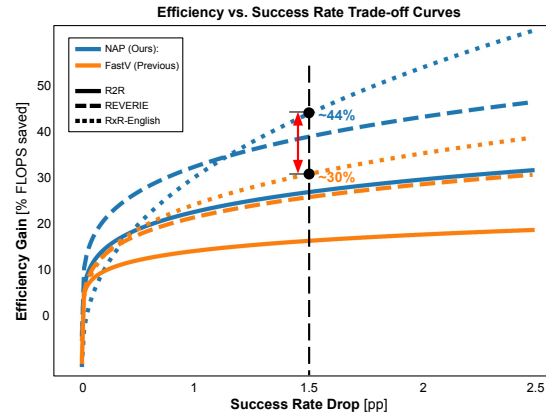
Figure 1: Efficiency-vs-Success-Rate trade-off curves for our method NAP (blue) and FastV (Chen et al., 2025) (orange) for 3 VLN datasets. Curves are fitted based on 15 token budget settings (100% to 30% of original budget). NAP consistently achieves greater efficiency for the same success rate loss compared to FastV. For example, for a 1.5% point (pp) drop in the success rate for navigation with RxR data, NAP achieves a 14% point gain in efficiency over FastV (red).
