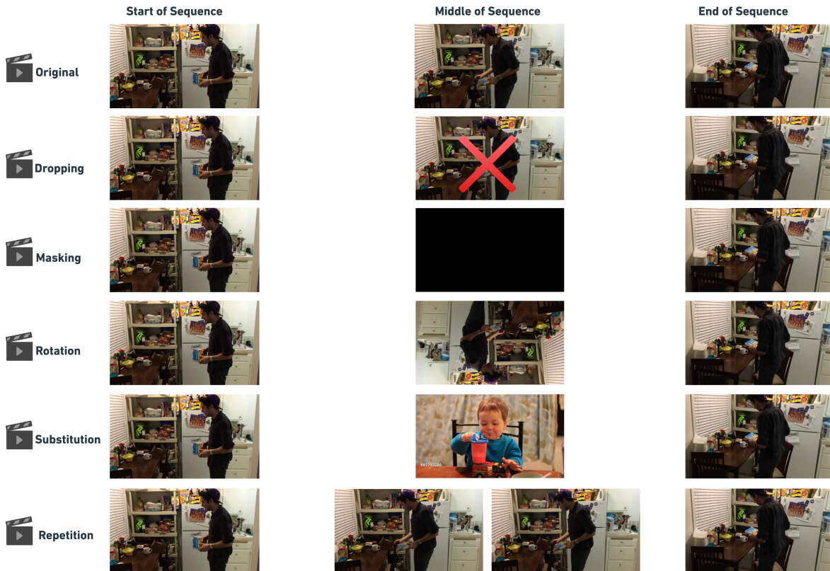
Figure 1: Illustration of the five video frame tampering techniques. Each row shows a specific tamper type applied to a video snippet, describing the respective impact on temporal/spatial coherence.
