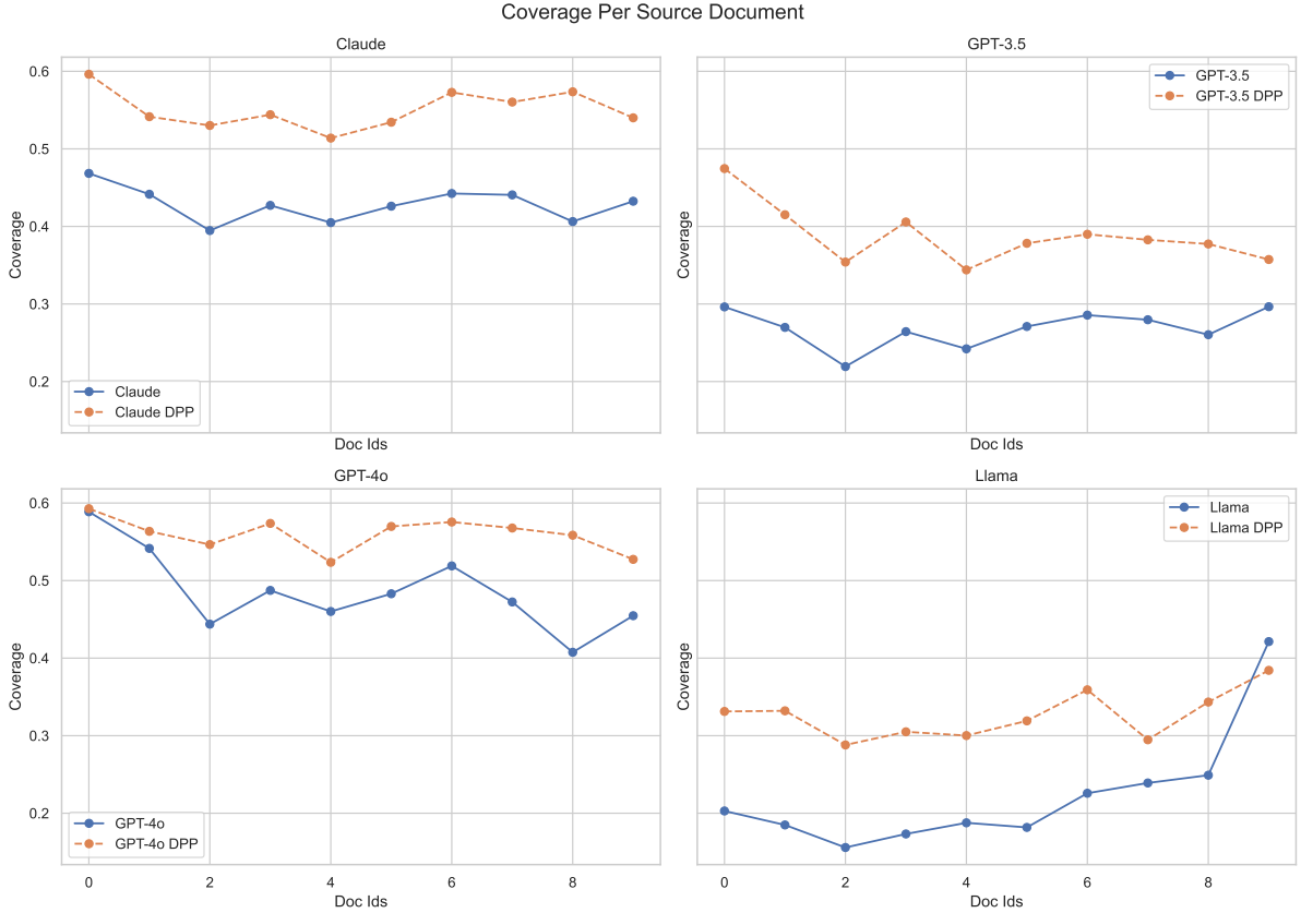
Figure 2: Studying the 'lost-in-the-middle' phenomenon by plotting coverage of different source articles by index with Naive LLM and LLM + DPP . While Naive LLM exhibits biases to better cover the articles at the start (GPT-4o, GPT-3.5) or end (Llama) of the context, LLM + DPP has higher and more uniform coverage of all source documents—mitigating these biases.
