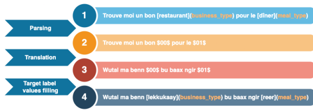
Figure 1: The three-step annotation projection algorithm: Parsing, which replaces the source annotations with ids, translation of the parsed sentence and backfilling of the translated annotations.
