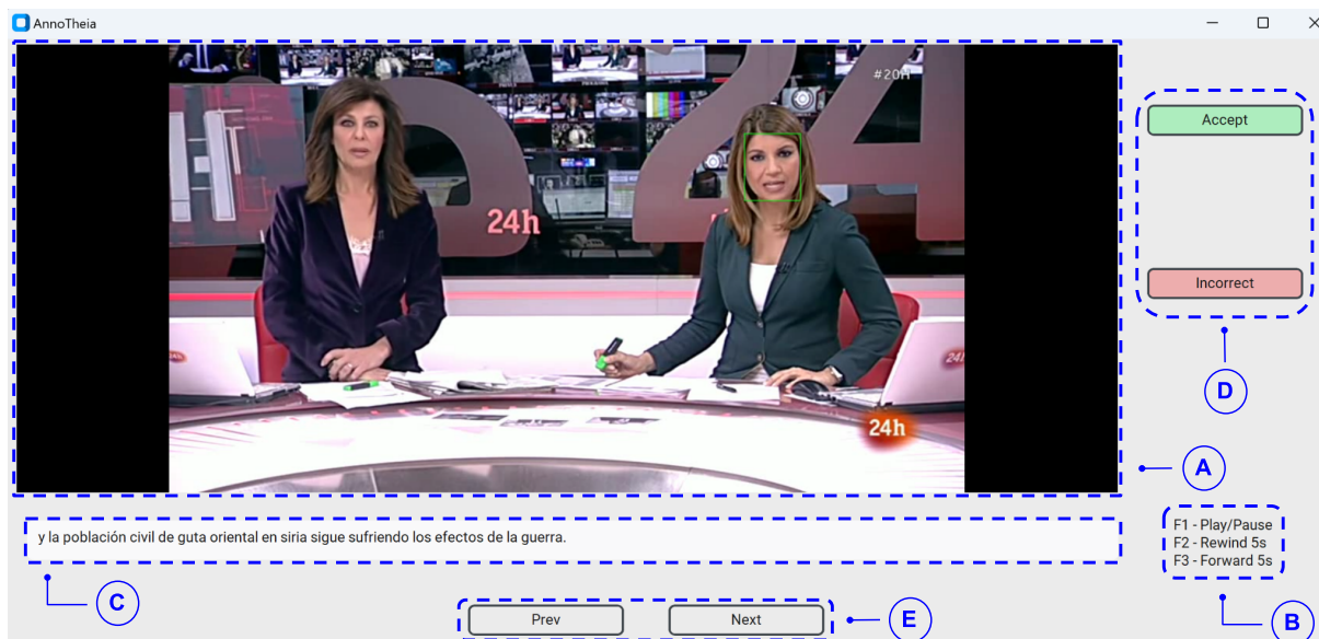
Figure 1: AnnoTheia toolkit user interface. A : Video display of the scene candidate to be a new sample of the future database. An overlying green bounding box highlights the active speaker detected by the toolkit. B : Keyword legend to control the video display. C : Transcription automatically generated by the toolkit. It can be edited by the annotator. D : Buttons to allow the annotator to accept or discard the candidate scene sample. E : Navigation buttons through candidate scenes. It can be useful to correct possible annotation mistakes.
