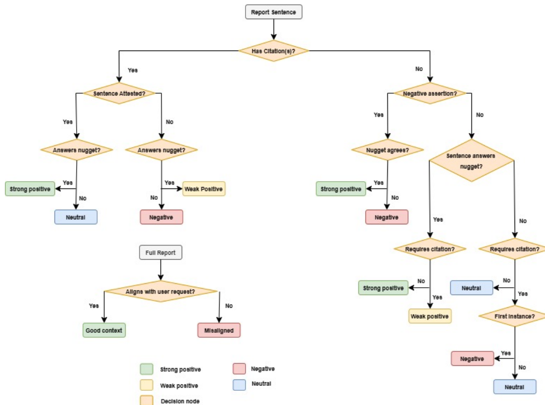
Figure 1: Adapted ARGUE decision tree for RAGTIME-1. The left subtree handles sentences with citations; the right subtree handles sentences without citations. The bottom section shows the report-level request alignment check, which applies a 0.7\times score multiplier to misaligned reports.
