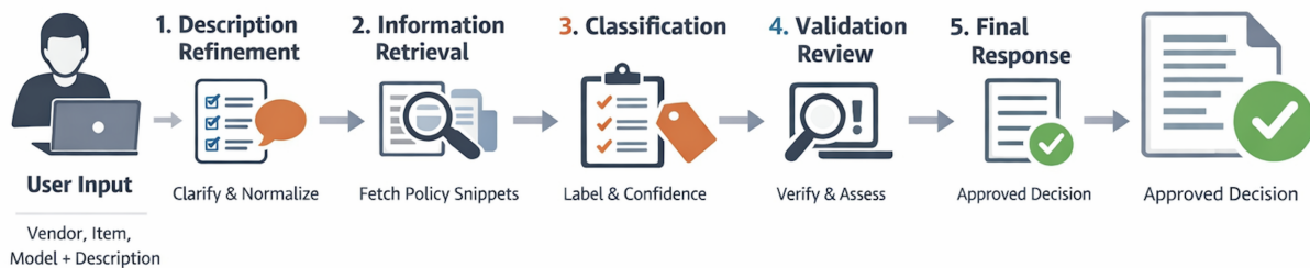
Figure 1: ORCHID Workflow: An SME inputs model, vendor, item and description of the asset; the system refines the property description, queries multiple policy databases, retrieves relevant information, classifies the asset, validates the classification and reasoning steps and produces the final response, which gets approved by the SME.
