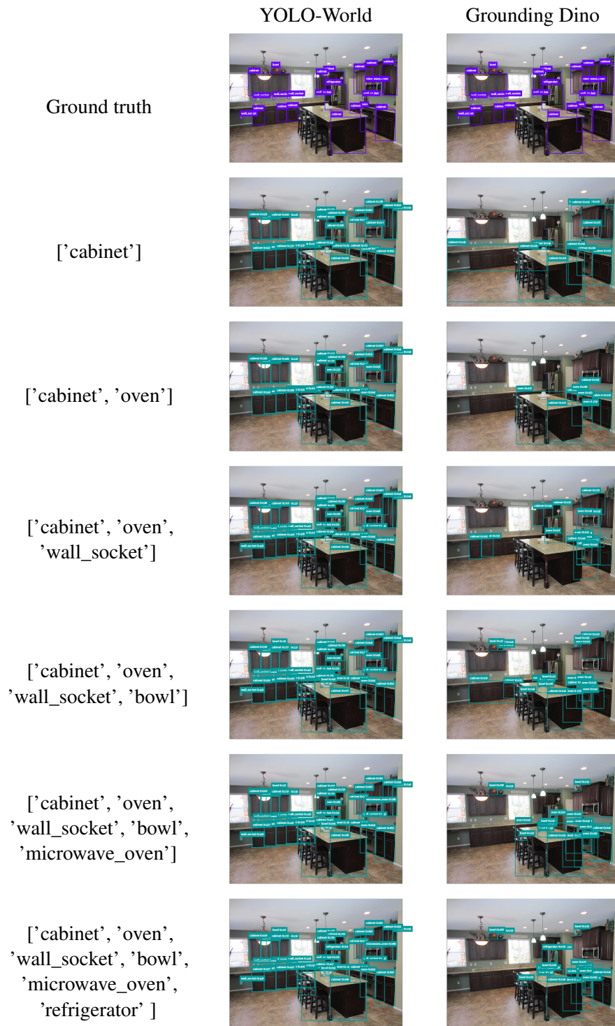
Figure 18: Subset of ground-truth classes evaluated with YOLO-World and Grounding Dino, illustrating how the models reassign object labels when it predicts higher confidence for an alternate class.
