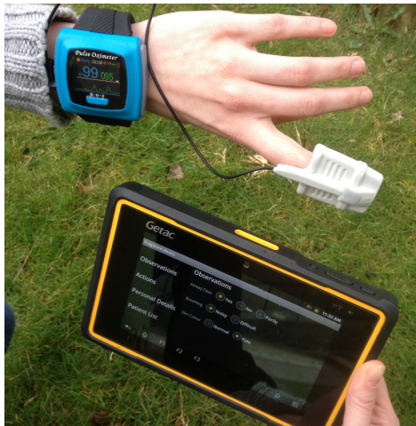
Figure 2: First hardware prototype of the MIME project (GETAC Z710 tablet and Pulse Oxymeter sensor).
