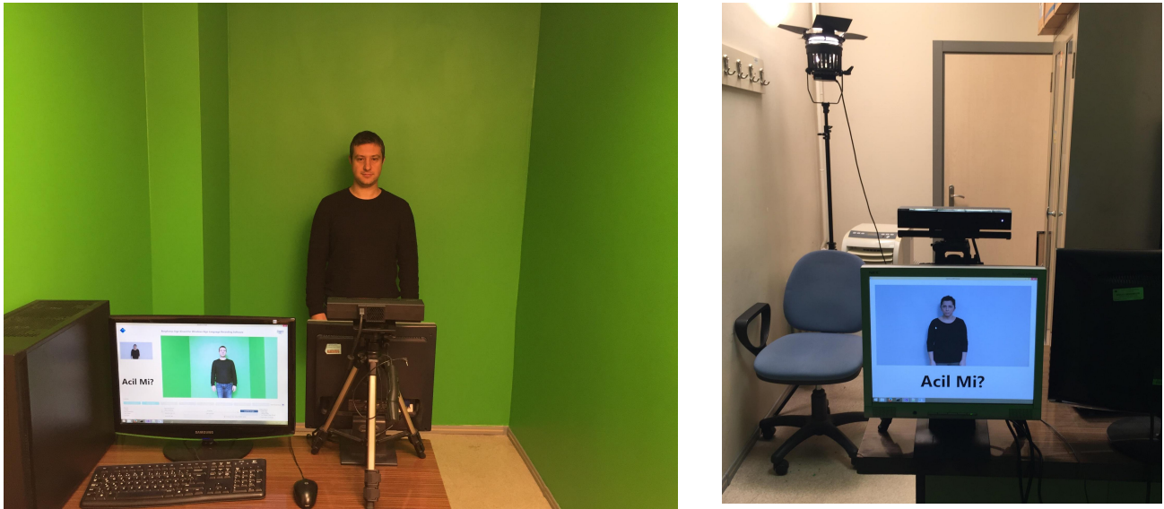
Figure 2: Recording Setup from the perspective of the user (Left) and the signer (Right)
