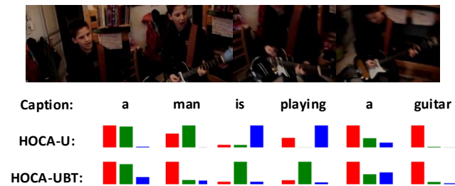
Figure 7: Visualization of the attention weights in multiple attentive fusion (MAF) module, the red bar denotes image modality, the green bar denotes motion modality, the blue bar denotes audio modality.
