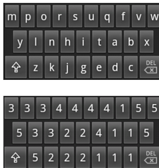
Figure 6: English keyboard optimized for both single finger and two-thumb input. This keyboard was generated with a population of 5000 over 20000 generations. This layout has an estimated typing speed of 82 WPM for two-thumb input and 27 WPM for single-finger input. There is an average distance of 1.46 keys between two characters in the same group. The lower diagram shows the group number of each character.
