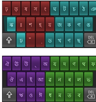
Figure 10: Optimized Assamese keyboard generated with a population of 5000 over 20000 generations. This layout has an estimated typing speed of 52 WPM and an average distance of 2 keys between two characters in the same group. The evaluated alphabetic groups are highlighted.
