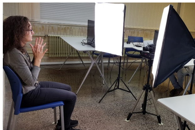
Figure 1: Set up of the dataset acquisition. Kinect and Nikon devices are rigidly mounted on a tripod at a fixed distance to the signer, that is uniformly illuminated over a somehow uniform background (location settings vary). No restrictions on clothing are imposed.
