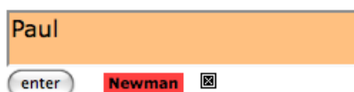
Figure 1: Interactive Machine Translation. Caitra uses the search graph of the machine translation decoder to suggest words and phrases to continue the translation.
