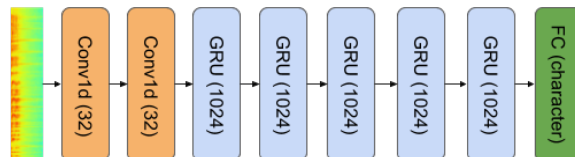
Figure 2: Architecture of the ASR model used in this work, following the DeepSpeech 2 architecture.
