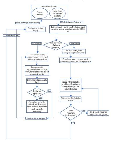
Figure 3: Flowchart for processing in the web tool
