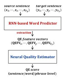
Figure 1: Two-stage Predictor-Estimator architecture (Kim et al., 2017).
