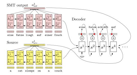
Figure 1: Illustration of a multiple-encoder sequence-to-sequence architecture as illustrated in Libovický et al. (2016).
