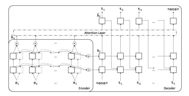
Figure 1: Schematic view of our MT network.
