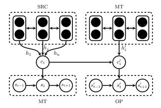
Figure 1: There are two bidirectional encoders that read the SRC and MT sequences. We maximize two training objectives: a translation objective (SRC  $\rightarrow$  MT) and a post-editing objective (MT  $\rightarrow$  OP). The OP decoder does a forced alignment with the MT encoder  $(t \rightarrow i)$ , and uses the corresponding global attention context  $c_i$  over SRC:  $c_i' = tanh(H_1c_i + H_2h_i' + b')$ . The MT decoder and MT encoder share the same embeddings.
